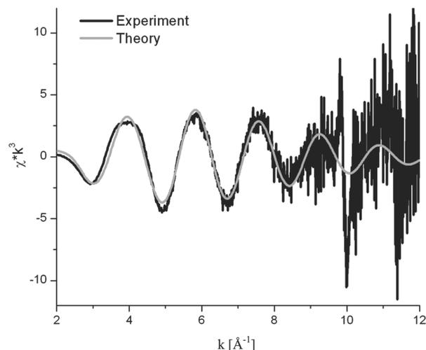
**Figure 2** EXAFS signal of a  $\sim 0.3$  mM Zn membrane transporter measured at 30 K with the Zn bent Laue analyzer (Mijovilovich *et al.*, 2004, courtesy of Professor J. Penner-Hahn, University of Michigan, USA).
