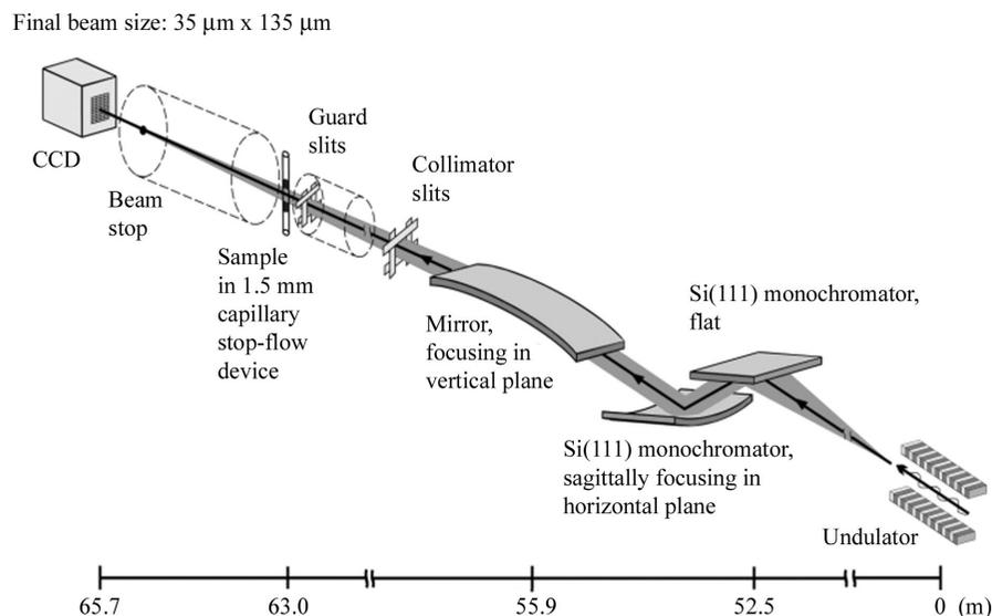
**Figure 1** Schematic drawing of the beamline optics. The X-ray beam travels from the right to the left in this figure. The second monochromator with the Si(400) crystals is omitted for clarity and is located at 53.5 m from the source. The experimental arrangement shown is for a standard 2 m SAXS camera with a flow cell for solution scattering. Spectroscopy experiments are performed on a remotely actuated table located approximately 61.5 m from the source (not shown).
