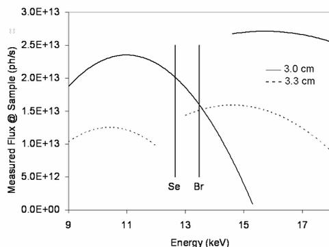
**FIGURE 2.** Comparison of the 3.3 and 3.0 cm period insertion devices. The Se and Br K-edges are indicated.
