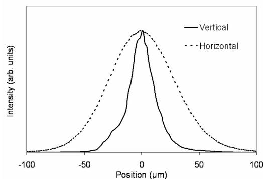
**FIGURE 5.** Beam profiles at the focal point. The vertical and horizontal beams measured 22.6 and 66.9  $\mu\text{m}$  FWHM, respectively.
